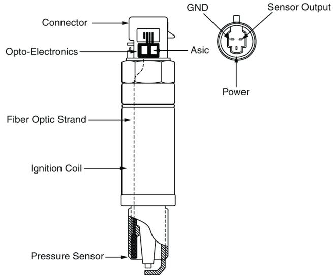
Fig. 5. PressureSense Igniter targeted for production engines
