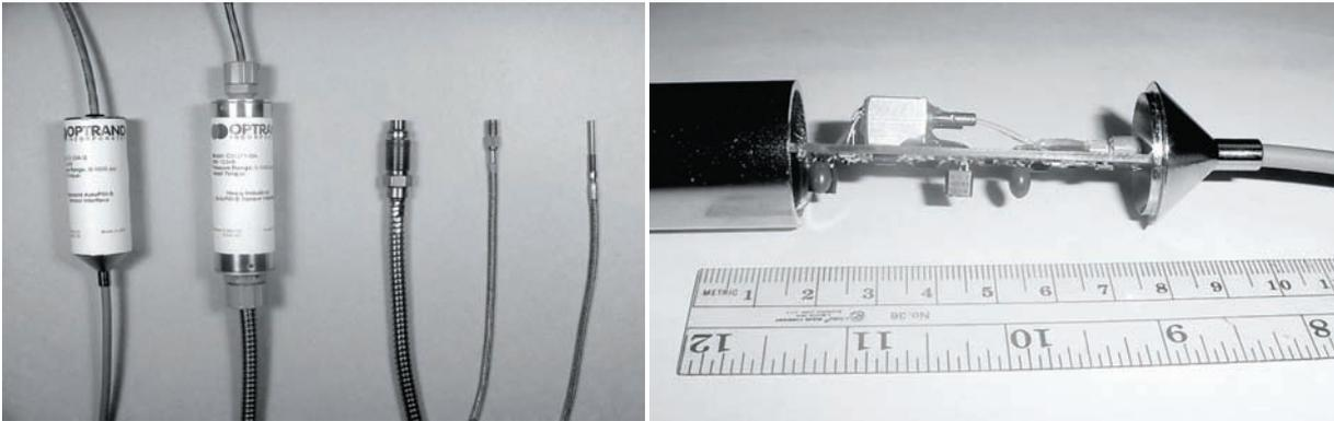
Fig. 3. Photographs of current cylinder pressure sensors used in engine R & D/monitoring
