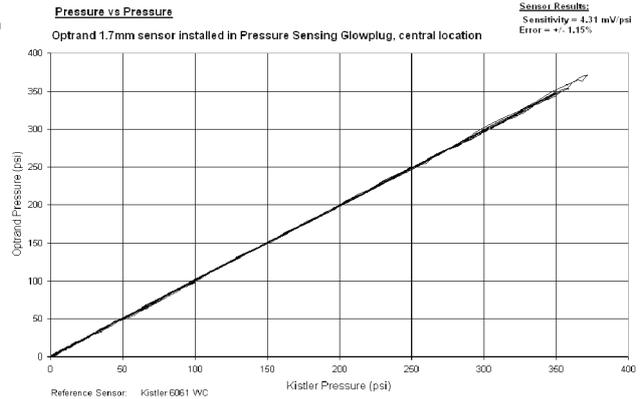
*Fig. 12b. Pressure vs. pressure comparison*
