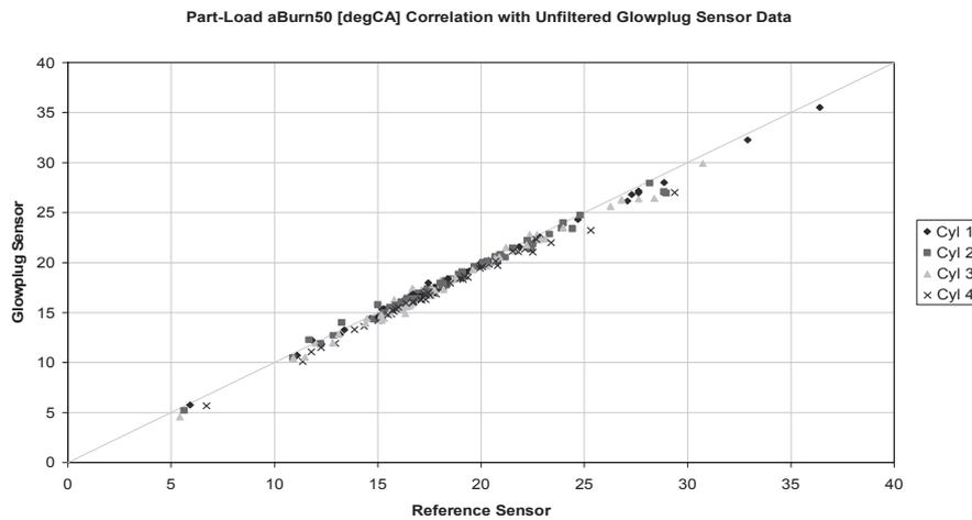
Fig. 13. 50% mass fraction burned comparison between PSGP and reference transducer
