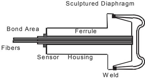
*Fig. 2. Sensor head construction*
