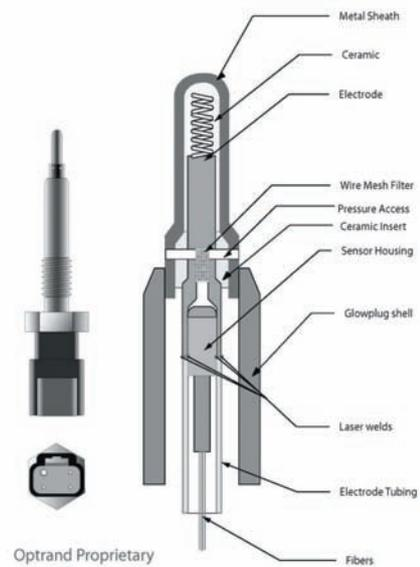
Fig. 8. PSGP targeted for use in production engines
