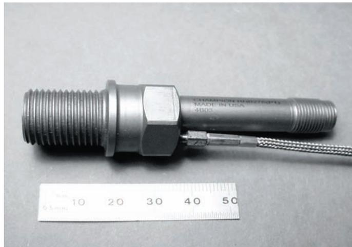
Fig. 6. PSIplug: Spark plug with removable sensor used in airplane engines
