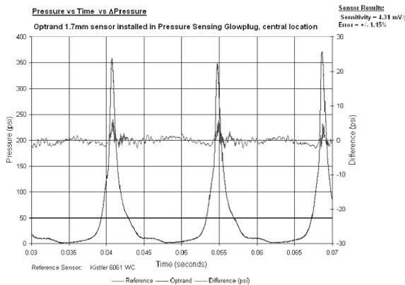
*Fig. 12a. Pressure vs. time performance comparison*
