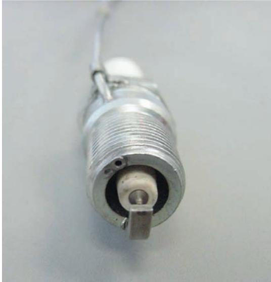
Fig. 4. Instrumented spark
