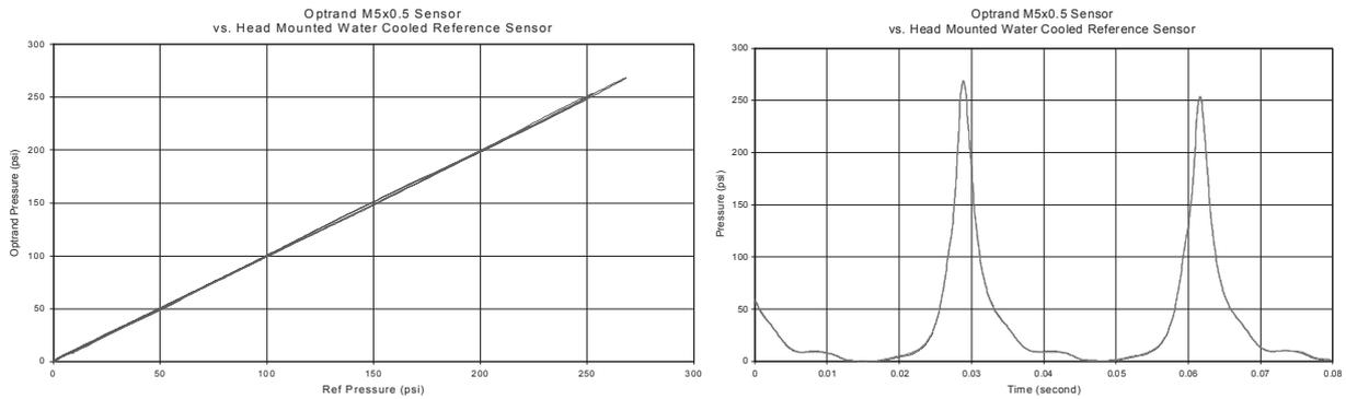
Fig. 9. Head-Mounted Sensor Performance: Total Non-Linearity\ Thermal shock +/- 0.44%
