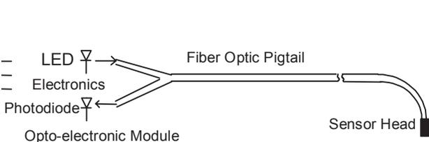
*Fig. 1. Schematic sensor construction*
