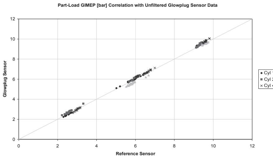
Fig. 14. IMEP comparison between PSGP and reference transducer
